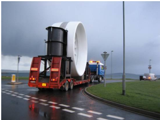
Transporting Open-Centre Turbine
